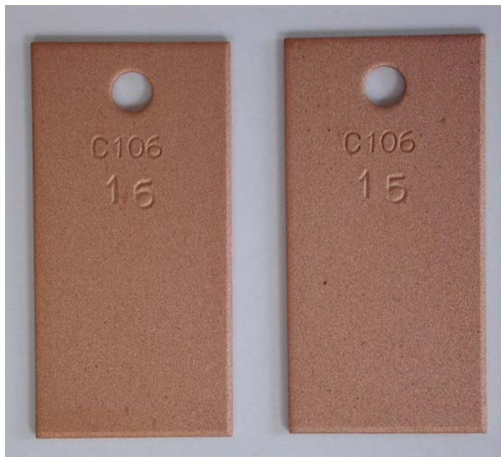
Figure 11 Copper Specimens –Soft Water Aerated
