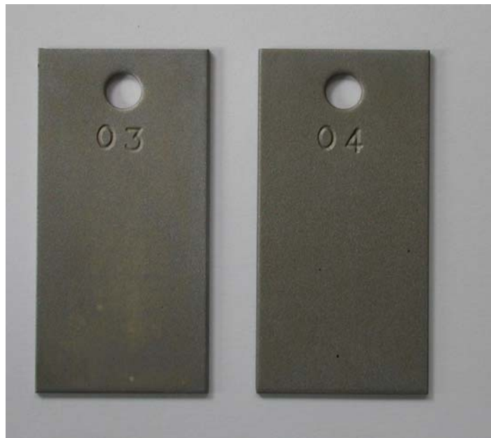
Figure 4 Steel Specimens –Soft Water Deaerated
